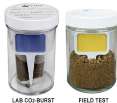
Figure 2. Jars and Gel Paddles for Solvita test. Photo courtesy of Solvita (solvita.com).
