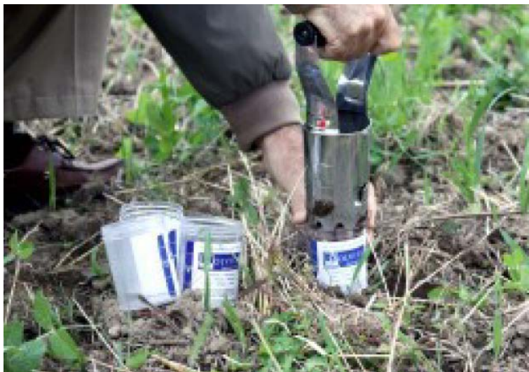
Figure 1. Collecting core samples for soil respiration test. Photo courtesy of Solvita (solvita.com).
