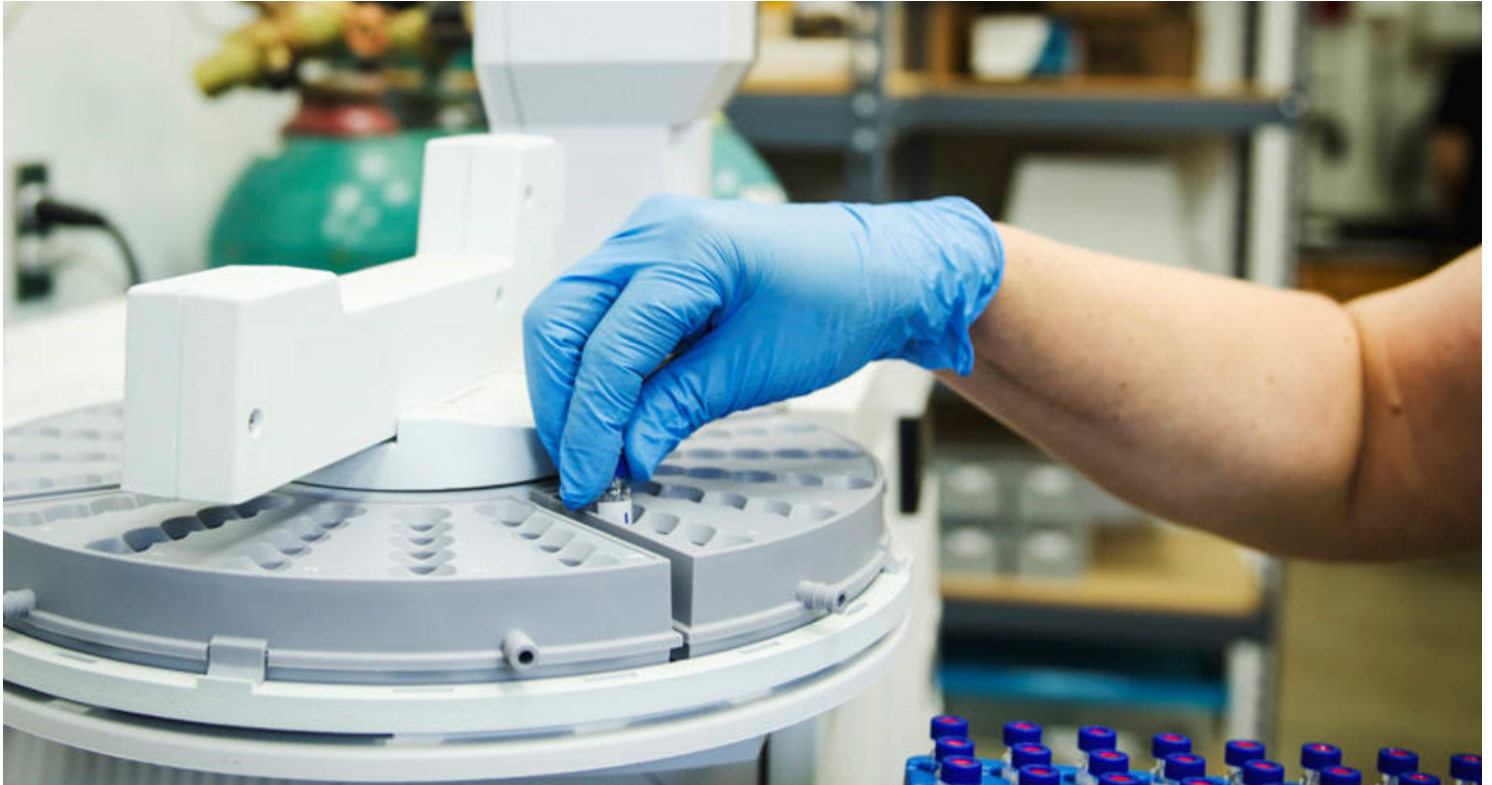
This gas chromatograph machine can measure the phospholipid fatty acid (PFLA) content of a particular soil sample. (University of Missouri)
